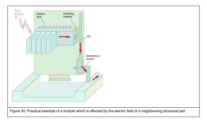
The disturbance voltage differences generate electric fields which act on the surface of the module. High-resistance networks with pull-up or pull-down resistors in the range of  $1 - 10 \text{ k}\Omega$  are especially sensitive to these electric fields. The connections of quartz crystal circuits, reset or all pull-up/pull-down arrangements are some practical examples.
