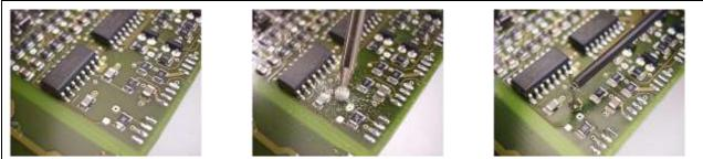
Figure 28: Prepare the ground layer by spot-facing, solder the contact pin in place, connect the generator cable to the contact pin with the micro-kleps and inject the disturbance current to ground via the conductor.
