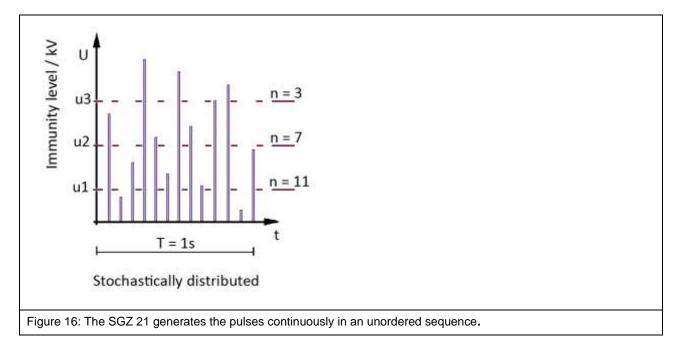
The generator and counter do not have to be synchronised. The start time does not affect the result. The number of pulses measured depends on both the device under test and the "Intensity" controller setting. The system works at its optimum if the greatest number of pulses does not exceed the value 2,000. The intensity should be reduced if necessary.
