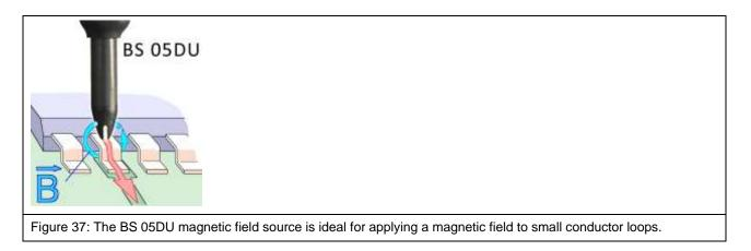
The magnetic field source with its field beam is guided directly across the module's surface for magnetic coupling (Figure 38). Only small surface areas are usually sensitive to magnetic fields. The field source has to be swivelled and turned to find these sensitive conductor loops with the field beam. Malfunctions are triggered as soon as a sensitive conductor loop has been found. Selected EMC measures can then be taken at this spot.
