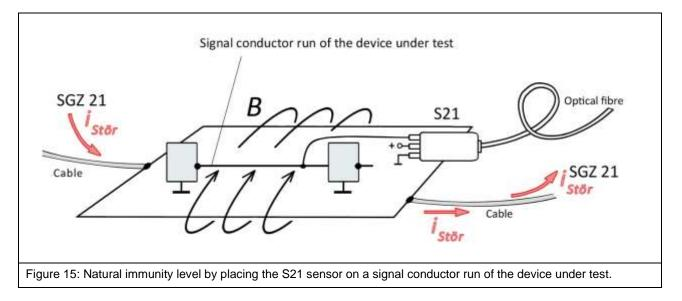
An original conductor run of the device under test is used for the same process in Figure 15. The pulse density method can be used with the set-up shown in Figure 13 if high-frequency signal sequences pass through this signal line.
