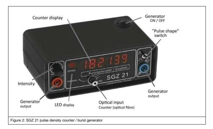
Generator ON/OFF: to switch the SGZ 21 on or off
