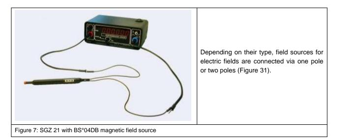
Apart from the field sources themselves, the connecting cables also generate fields that may couple to the device under test and affect the measurement result. Cables should thus always be kept away from the device under test if possible.
