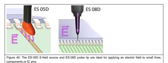
The electric field source with its field is guided directly across the module's surface for electric coupling (Figure 41). Only small surface areas are usually sensitive to magnetic fields. The field source is gradually moved towards the sensitive area on the module. Malfunctions are triggered as soon as a sensitive area has been found. Selected EMC measures can then be taken at this spot.
