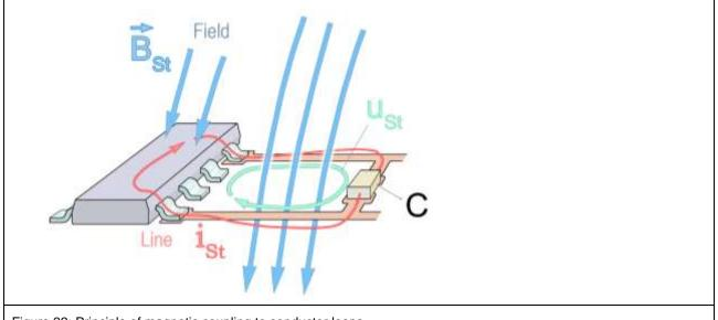
Figure 32: Principle of magnetic coupling to conductor loops.
