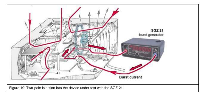
Both generator outputs are connected to the device under test for two-pole coupling.
