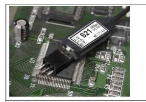
Figure 9: S21 sensor connected to an IC in the device under test, for example, via a three-pole socket.
