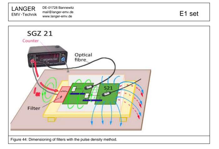
Dimensioning of filters is a typical use of the pulse density method (Figure 44): The SGZ 21 is used to inject a disturbance current into the device under test. The S21 sensor establishes the device's immunity level with a line of the device under test and transmits a signal to the SGZ 21's "counter input" via an optical fibre each time the level is exceeded. A high value indicates a sensitive line which is sensitive to disturbances.
