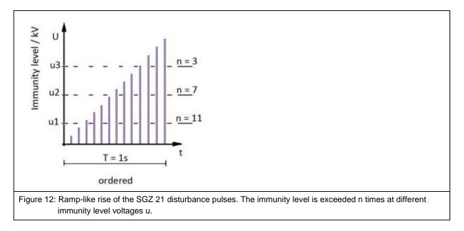
Figure 12 shows how the pulse density method functions in principle. The voltage u of the disturbance pulses gradually rises from a minimum value to a maximum value up a ramp over the time T = 1 s. This process is continuously repeated.
