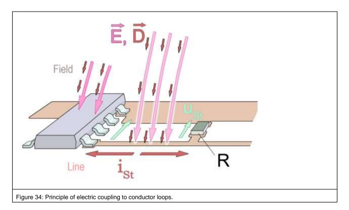
The coupling electrode formed by the conductor run has an outer capacitance per unit length which is the total capacitance  $C_P$ . This capacitance absorbs a displacement current i(t) from the electric field and feeds this to the conductor run.
