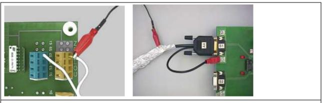
Figure 23: The generator is connected directly to control and auxiliary power lines. With data lines, the generator pole is connected to the line shielding or a capacitor coating.
