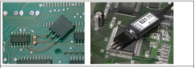
Figure 43: A socket where the S21 sensor can be connected is stuck on the printed circuit board.
