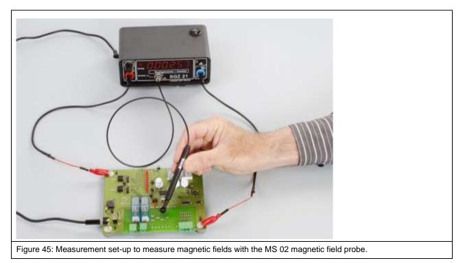
The disturbance current which is fed into the module distributes according to the module's metallic system. The ground system usually accounts for the largest share of the metallic system. This means that the disturbance current will flow via the ground system and the respective magnetic field depends on the form of the ground system. Figure 46 shows the current flow and the respective magnetic field.
