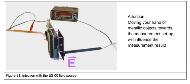
The E-field source (ES 00 to ES 02) connected to the SGZ 21 is used to simulate the neighbouring metal system which generates the electric field (Figure 31). The size of the E-field source can be selected based on
