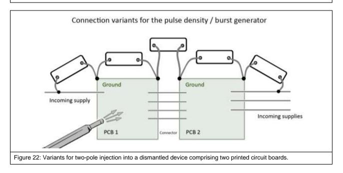
The printed circuit boards of the device under test are now fully accessible and disturbance current can be selectively coupled to them via a two-pole connection.
