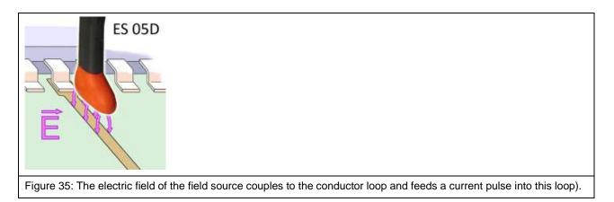
In the process of interference suppression with field sources, the electric field is generated by the field source. The field source must be held so that its field acts on the sensitive conductor run/component. The closer the field source is brought to the conductor/component, the more intensive is the interference.
